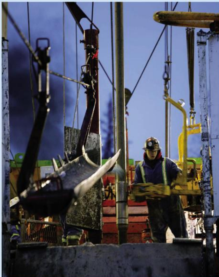
First Choice Pipehandlers laying down pipe at a rig site south of Grande Prairie.
